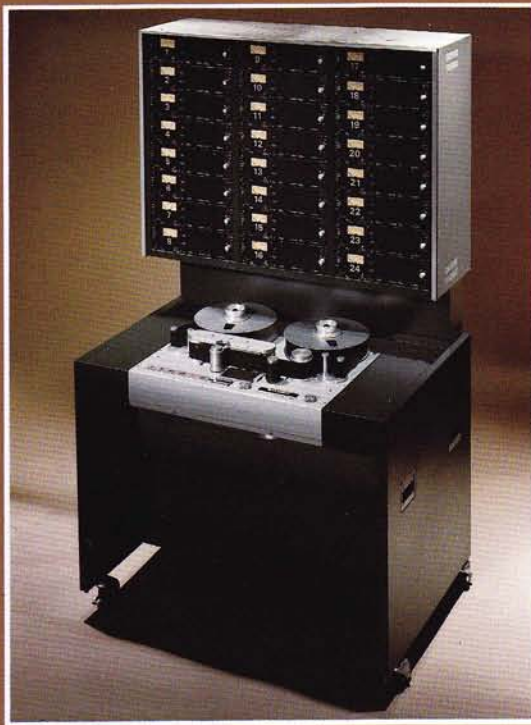
STUDER A80VU-24-2" MK III twenty-four track, 2" tape width
